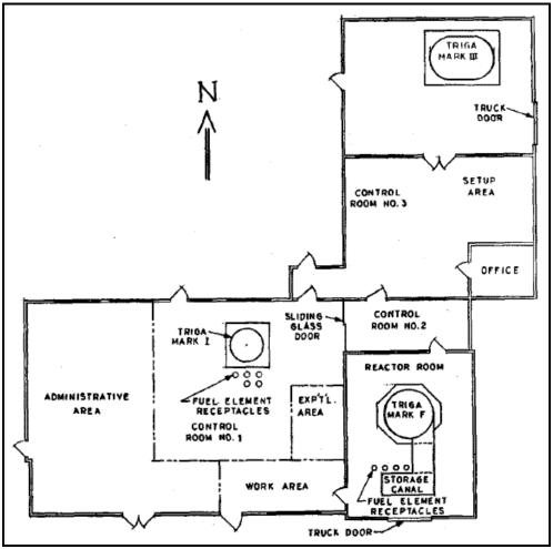
Figure 2-9. Plan view of TRIGA Reactor Facility (GA 1969).
