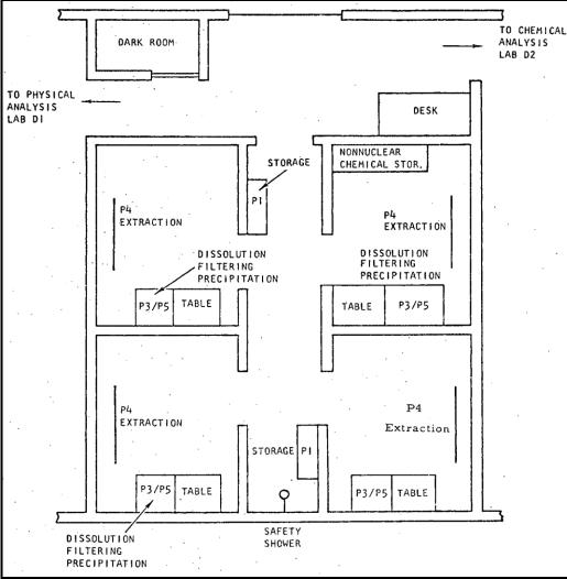
Figure 2-6. Uranium Purification Area (SNM-696, p. 205).
