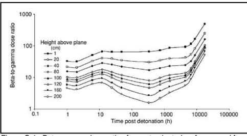
Figure C-1. Beta-gamma dose ratios for contaminated surfaces used for Pacific tests (Barss 2000).
