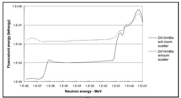
Figure A-9. Lethargy neutron spectra for an <sup>241</sup>AmBe calibration source with and without room scatter (IAEA 2001).
