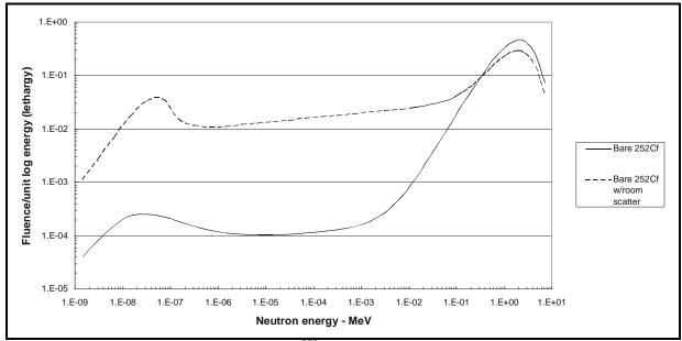
Figure A-7. Lethargy neutron spectra for <sup>252</sup>Cf calibration source with and without room scatter (IAEA 2001).
